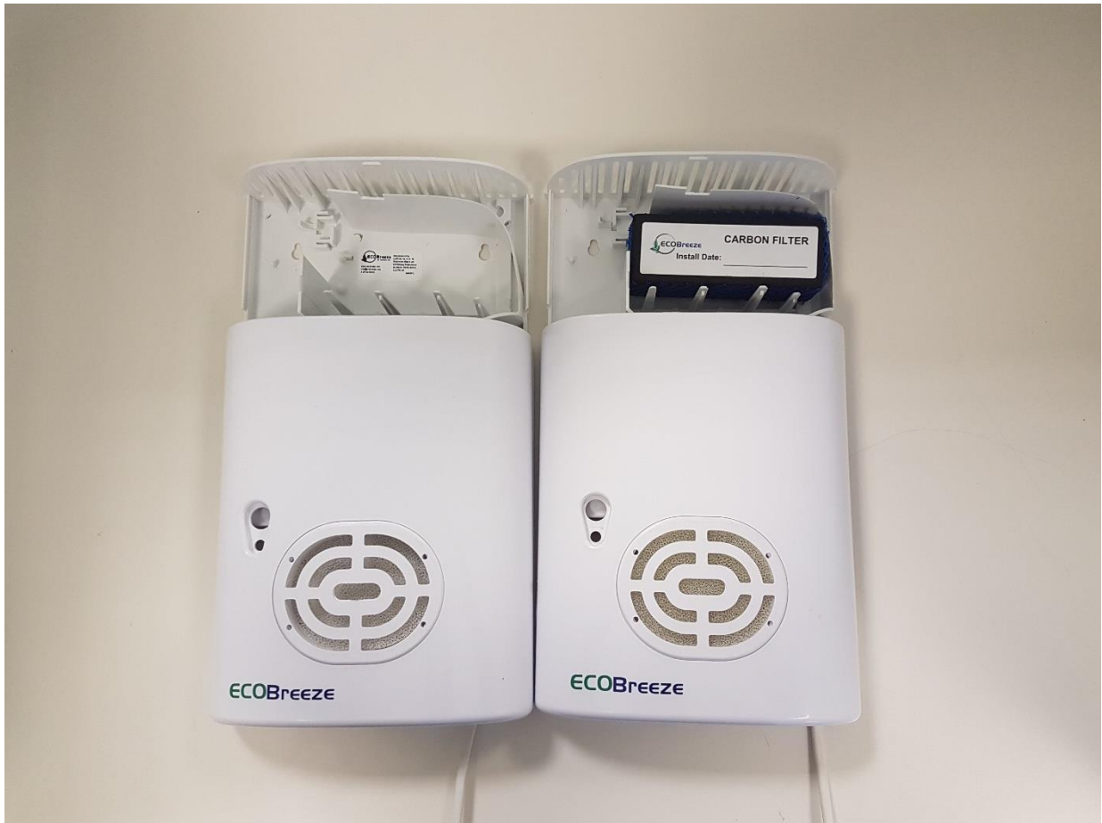
Figure 5: Photograph of opened Ecobreeze unit with and without carbon filter fitting (unit was closed for testing)
