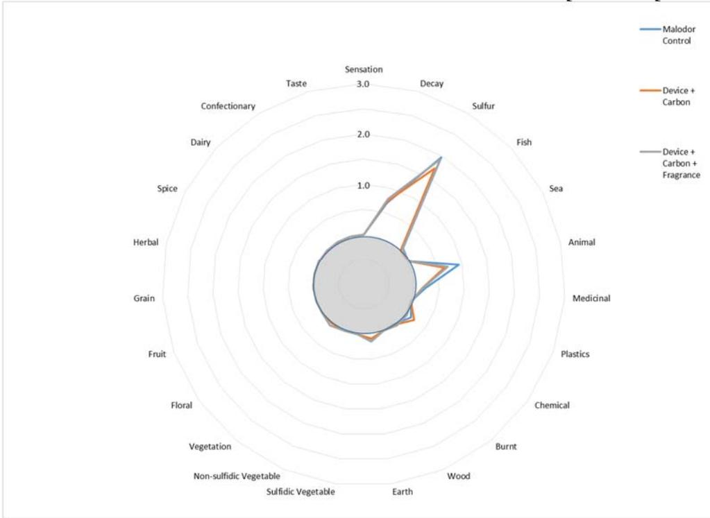
Figure 6. Odor character profile at 30-minutes for all samples during fecal malodor reduction test. The results of the Ecobreeze device with carbon are the means of two replicate samples.
