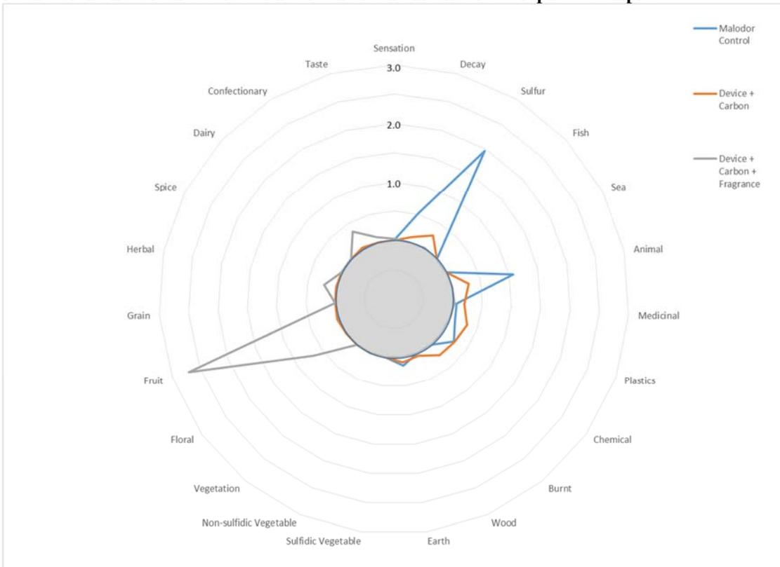
Figure 8. Odor character profile at 2-hours for all samples during fecal malodor reduction test. The results of the Ecobreeze device with carbon are the means of two replicate samples.
