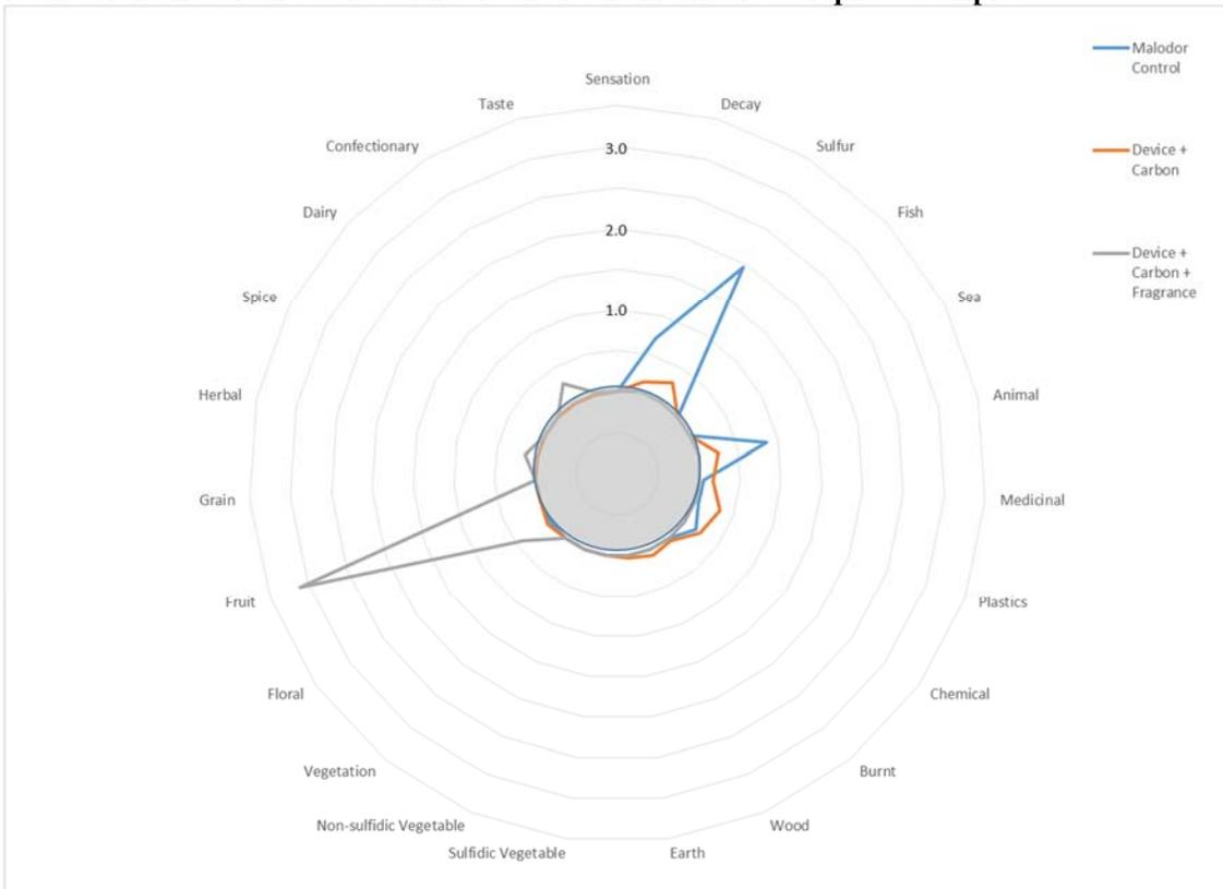
**Figure 10. Odor character profile at 4-hours** for all samples during fecal malodor reduction test. The results of the Ecobreeze device with carbon are the means of two replicate samples.
