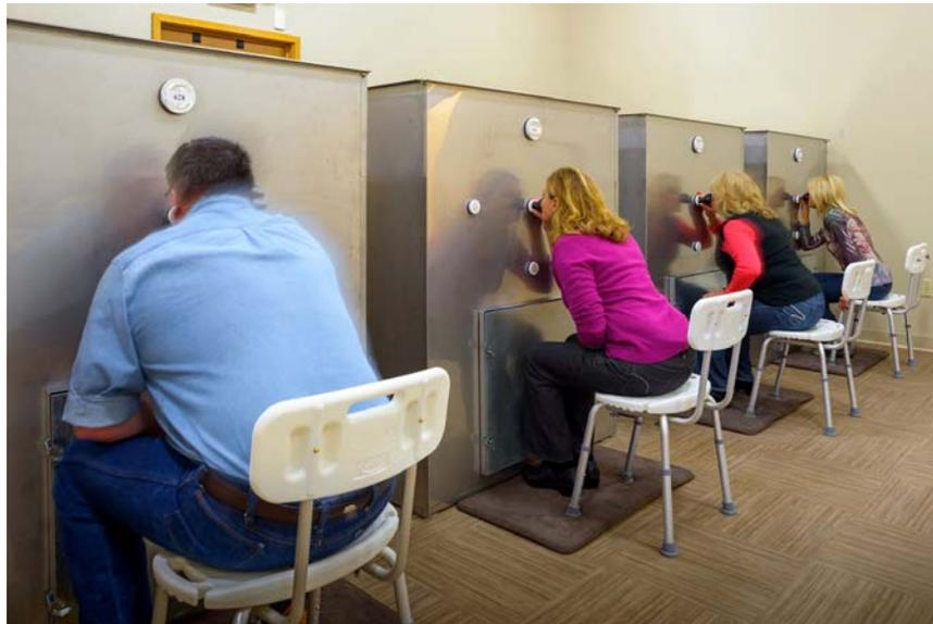
**Figure 1. Four of the stainless steel chambers utilized for malodor reduction efficacy testing at St. Croix Sensory, Inc. The chambers are all identical 1.2x1.2x1.5m boxes with a sniffing port in the center on the front, multiple testing ports also on the front, two access and exhaust ports on the top, and an access hatch on the front. An exhaust system on top of the chambers is used to purge the chambers at the end of each test.**
