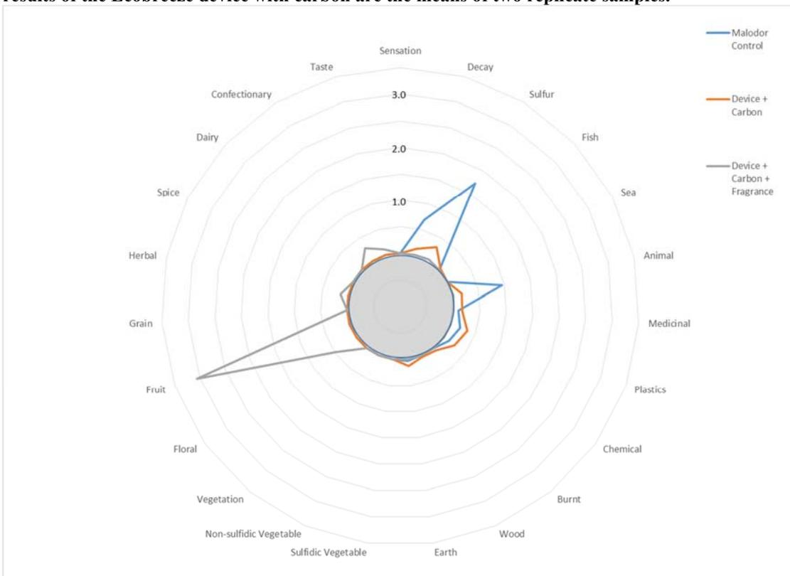
**Figure 9. Odor character profile at 3-hours** for all samples during fecal malodor reduction test. The results of the Ecobreeze device with carbon are the means of two replicate samples.
