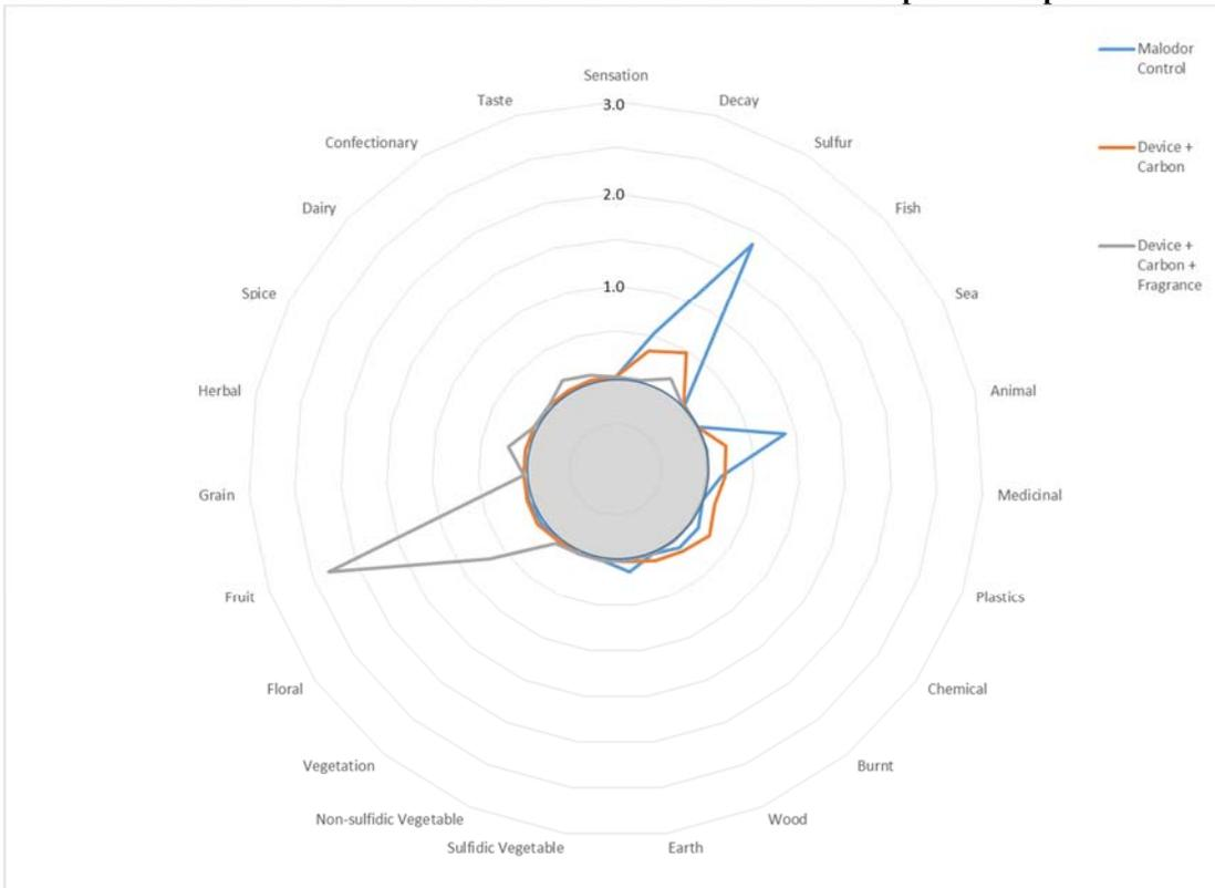
Figure 7. Odor character profile at 1-hours for all samples during fecal malodor reduction test. The results of the Ecobreeze device with carbon are the means of two replicate samples.
